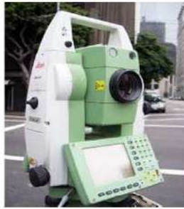
Leica TCRA 1201 Robotic Total Station
