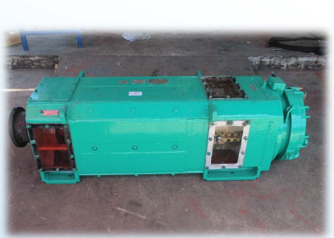
DC Motor 37 KW
