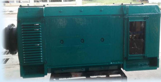
DC Motor 120 KW
