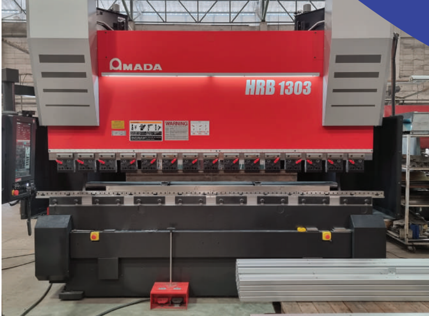
Amada HRB 1303 Hybrid Press Brake Bending Machine Bendable length upto 3 meters
