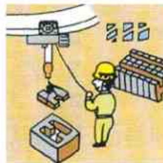
Accurate positioning (The hoisted load does not shake.)
