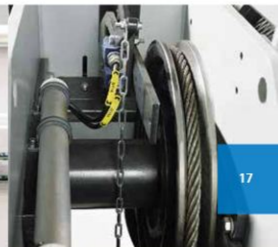
Free accessible pulleys and hook operated ultimate hoisting limit switch
