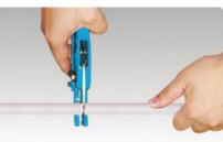
Cut the pipe vertically and clean the cutting head.
