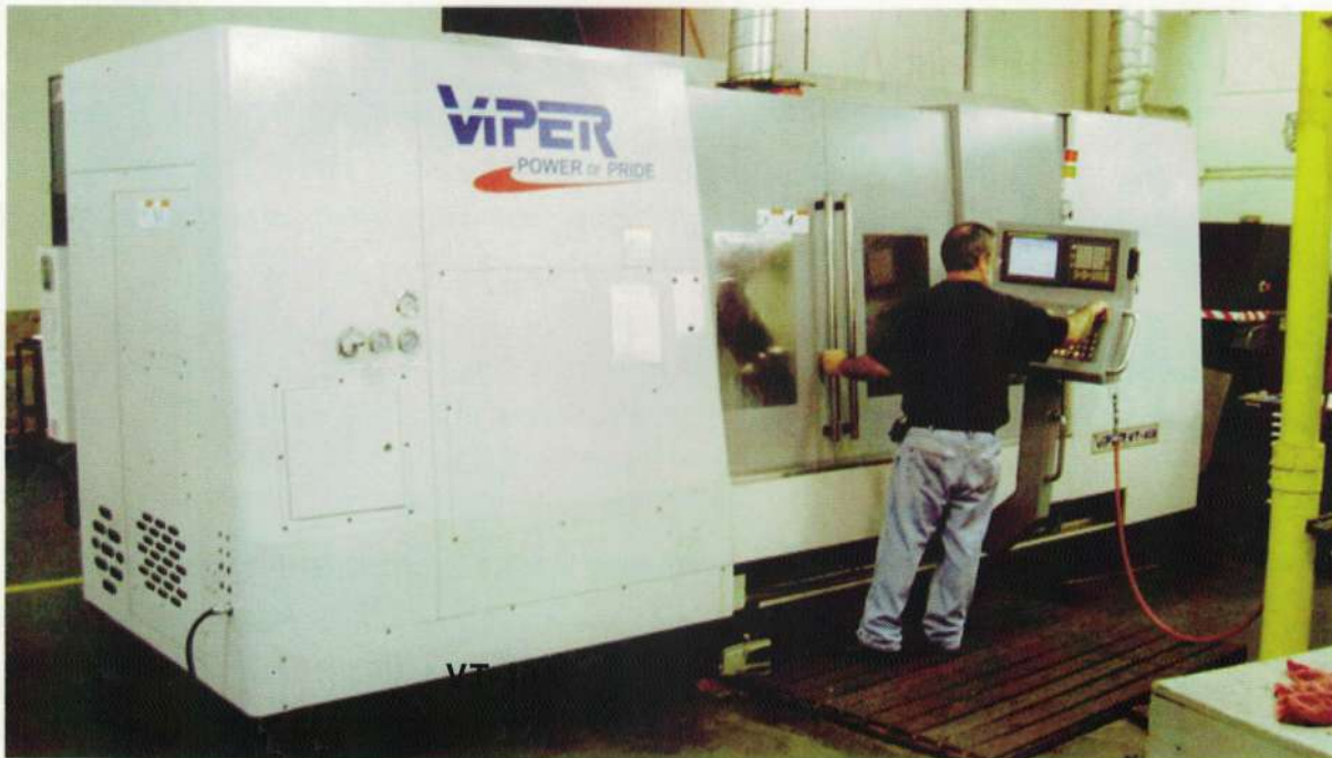
Milling a landing gear component on a Mighty Viper Lathe with TP2500 CNMG 643W-MR7 chipbreaker insert at V&M.
