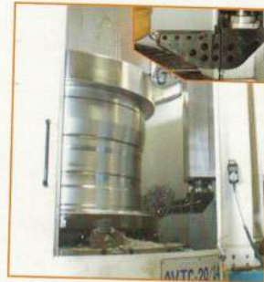
VTL-Series turning a Drive Roll workpiece from 43,000 lbs. stock cylinder blank – L-Type tool holder.
