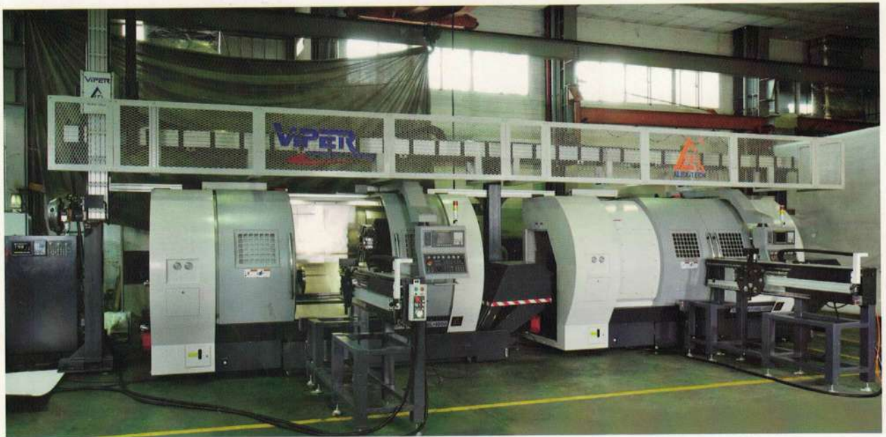
Application example: VT-36B with automated parts loading and unloading.
