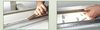
A Shine Co. craftsman performing precision hand scraping, our guarantee of high precision.
