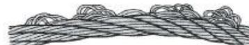
Protruding Core because of shock loading, torque build-up during installation, tight sheaves, or incorrect rope design.
