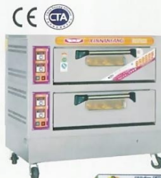
Luxury Gas Oven (3 Decks 6 Plates) Model:ET-NFR-60H W1480xD1130xH1830mm Volt:220V/50Hz Power:300W Power:79,845BTU/hr Temperature:20~400°C N/W:613kg
