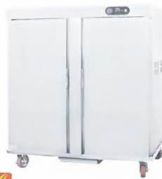
Food Warmer Trolley With Double Door Model : ET-DH-22-21 W1540xD940xH1795mm Bore Dimensions: W1350xD680xH1380mm Volt:220V/50Hz Power:2.62KW Capacity:22 Layers N/W:320kg
