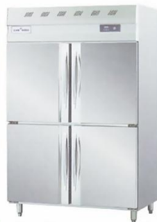
4 Door Commercial Freezer Model: ET-1.0LG-4 W1220xD780xH2050mm Internal Dimensions:W1100xD630xH1460mm Volt:220V/50Hz Power:0.65KW Capacity:1010L Temperature:10~-18°C N/W:200kg
