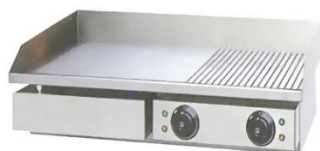
Electric Griddle (1/2 Grooved) Model : ET-TEG-822 W730xD500xH220mm Volt:220V/50Hz Power:4.4KW N/W:38kg
