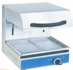
Electric Salamander Model : ET-TES-450K W450xD450xH500mm Volt:220V/50Hz Power:2.8KW N/W:38.5kg
