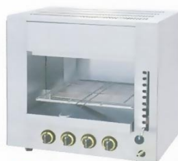
Gas Salamander Model : ET-TGS-14 W620xD440xH610mm Power:23,885BTU/hr N/W:41kg
