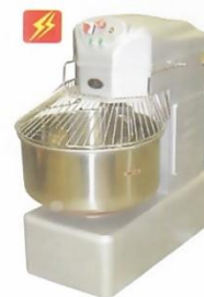
Spiral Mixer Model:ET-HS20S W710xD500xH780mm Volt:220V(380V)/50Hz Power:0.75KW N/W:142kg Drum Volume:23L Max Flour Load:8kg
