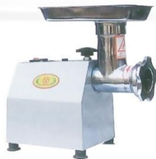
Electric Meat Mincer Model : ET-MM-8 W345xD190xH355mm Volt:220V/50Hz Power:0.4KW Out Put:80kg/hr N/W:16kg
