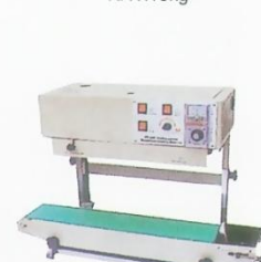
Vertical membrane Sealing Machine Model : ET-FR-150V Size : 850x420x360 mm Power : 500W Voltage : 220V/50Hz Sealing speed : 0~13 m/min Sealing Width : 6-15 mm Temperature Range : 0-300 °C
