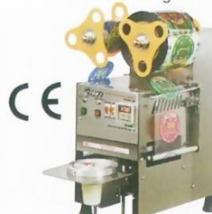
Stainless Steel Fully Auto Sealing Machine Model : ET-Q9 Size : 282x370x540 mm Power Supply : 220V/50Hz Power : 360W Out Put : 300~400 cup/h N/W:28kg
