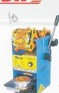
Semi-auto Sealing Machine Model : ET-B7 Size : 205x265x460 mm Power Supply : 220V/50Hz Power : 315W Out Put : 300~400 cup/h N/W:15kg
