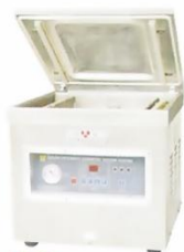
Semi-automatic Vacuum Packager Model : ET-DZ-400T Size : 540x490x530 mm Power : 750W Power supply : 220V/50Hz Exhaustment of pump : 20m3/hr Vacuum pressure : 0.66KPa Machine Weight : 102kg
