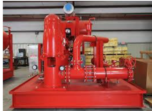
Vertical Turbine Diesel Fire Pump
