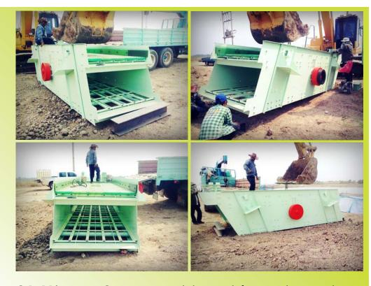
SiL Vibrating Screen is widely used for grading and screening materials in the fields of minerals, quarry, building materials, etc. Our vibrating screen has multi-layers and its screen size is various, it can screen out many kind of materials with different size.
