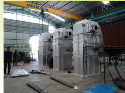
Bucket Elevator SUS304
